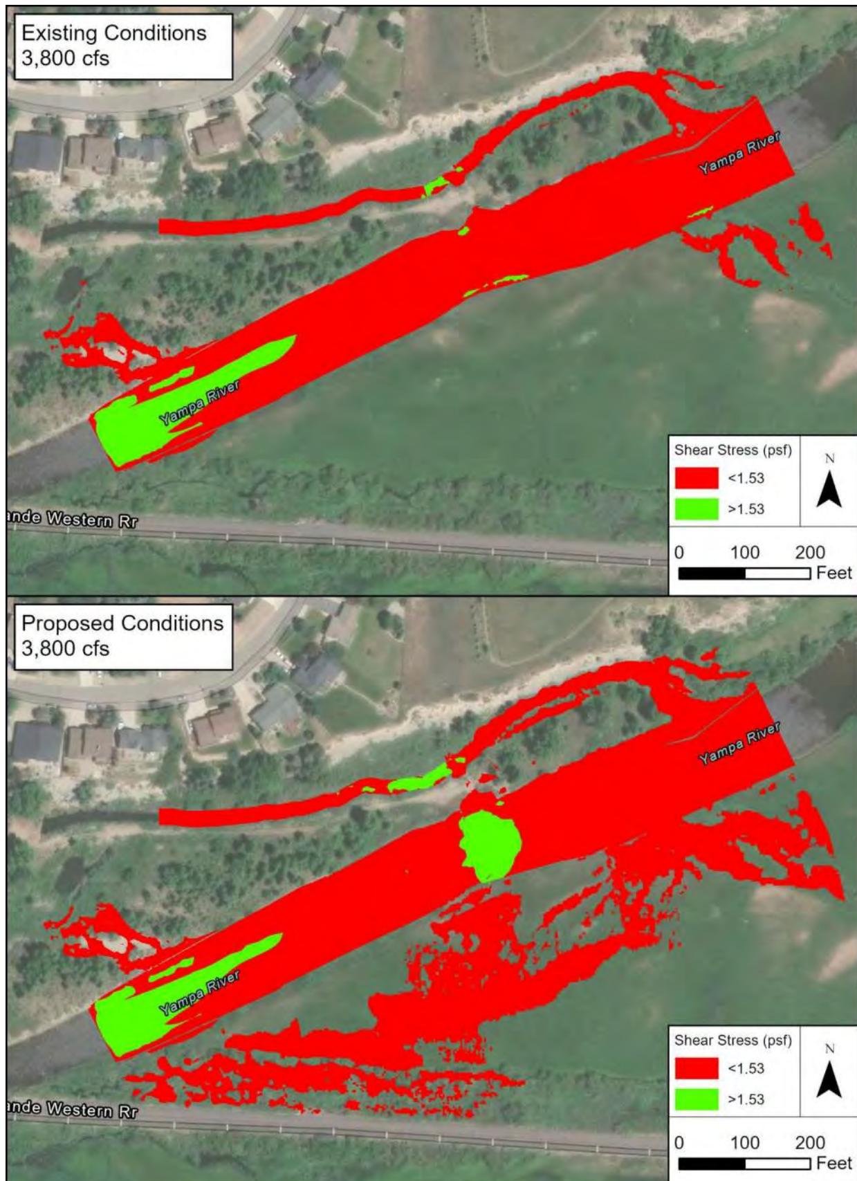
Figure 23: Incipient Motion Analysis - 3,800 cfs
