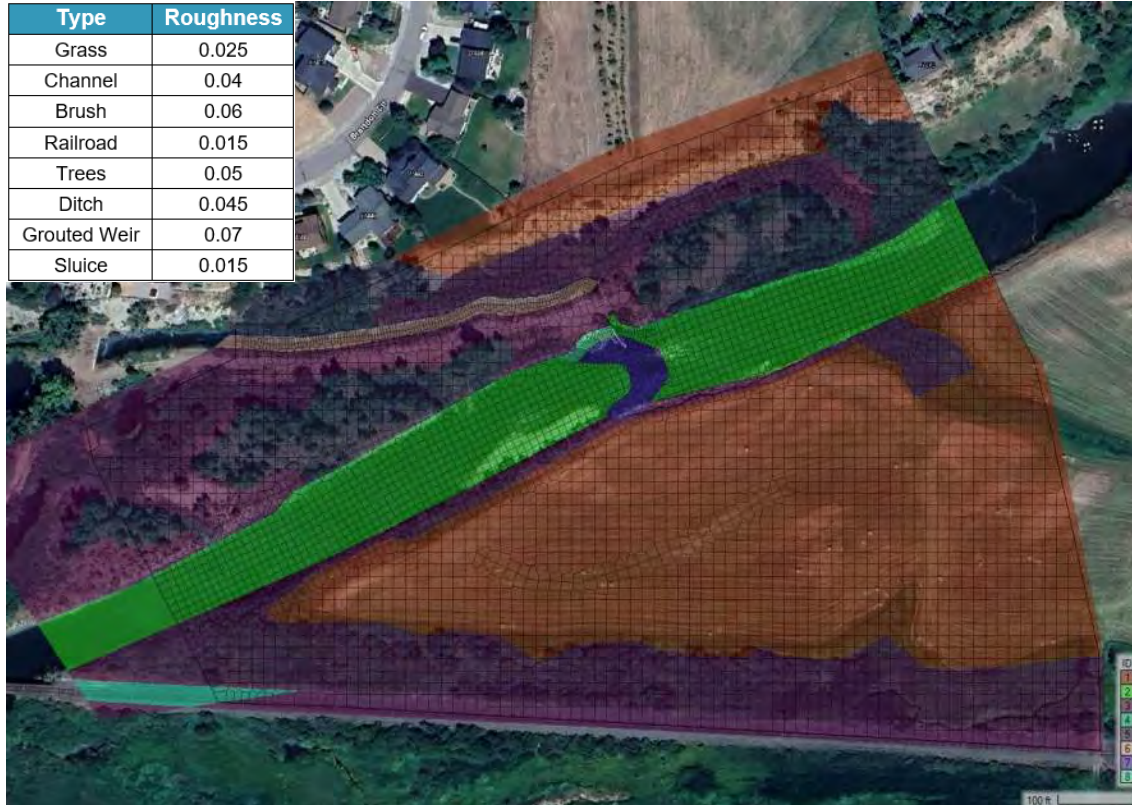
Figure 13: Close-up View of the 2D Model Mesh Surrounding the Proposed Whitney Ditch Diversion Structure
