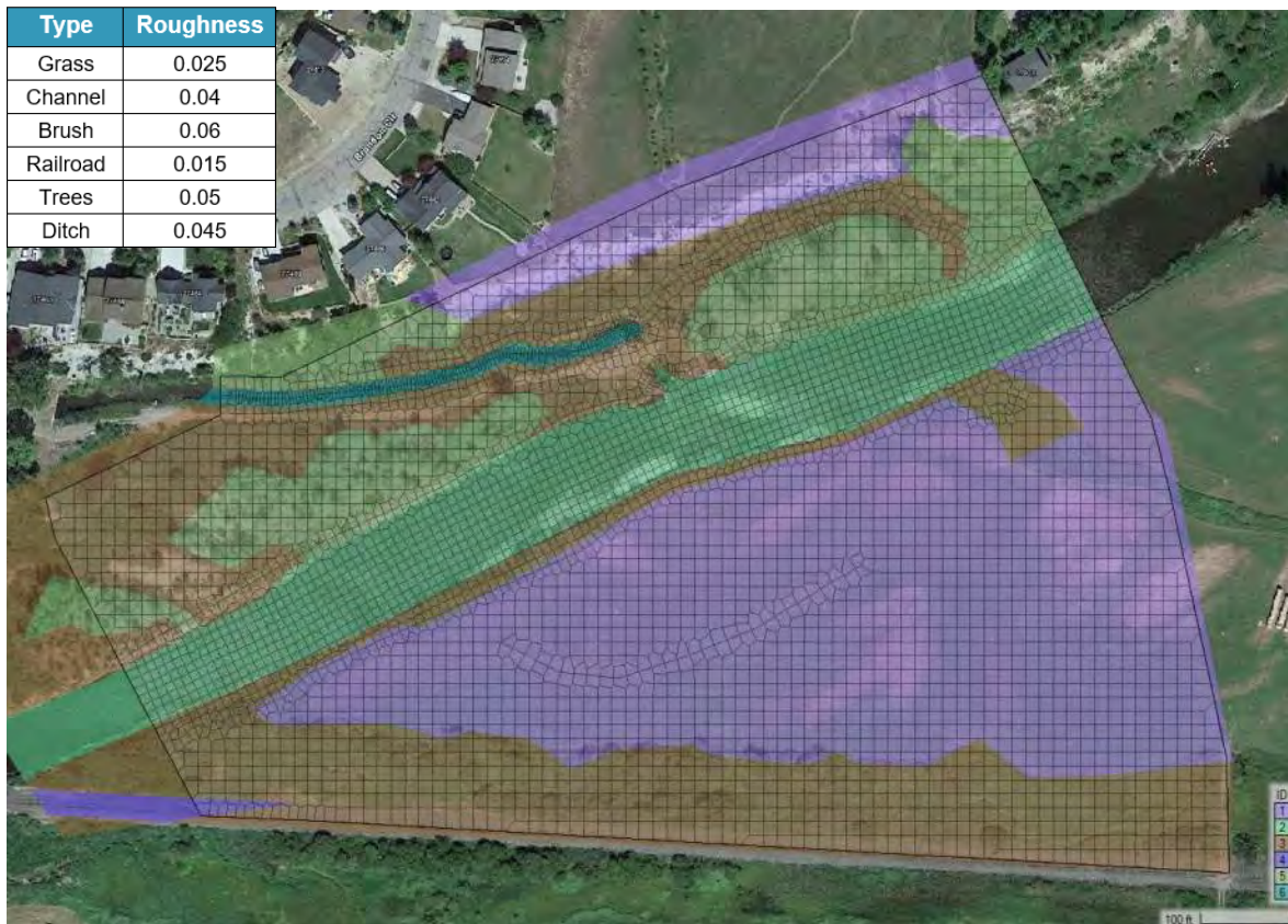
Figure 11: Manning's n Roughness Zones and Values for the Existing Conditions 2D Model
