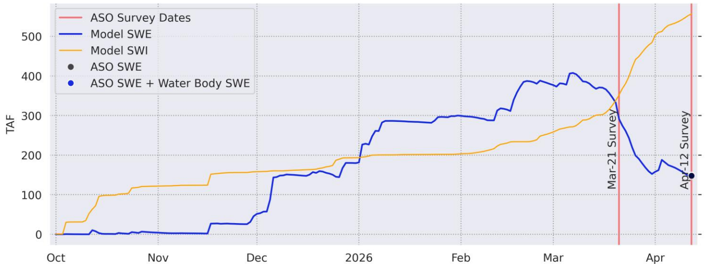
Figure 3. Daily timeseries of modeled SWE volume (TAF) and Surface Water Input (SWI) volume (TAF) for the Yampa and Elk Rivers. In this instance, the ASO SWE (black dot) and the ASO SWE + Water Body SWE (blue dot) are overlapping.
